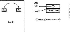
Flange should be at least 3 inches wide. Score so flap will bend up to allow wire to be threaded.
